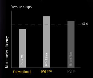
The innovative HVLP<sup>Plus</sup> nozzle air head system guarantees substantial material savings plus an outstanding surface finish. Tests by the Fraunhofer IPA according to EN standard 13966-1 with an HS-2K top coat resulted in transfer efficiencies of up to 88%. This puts the transfer efficiency far above the 65% required for HVLP applications - that way the PILOT Premium pays for itself in next to no time.
