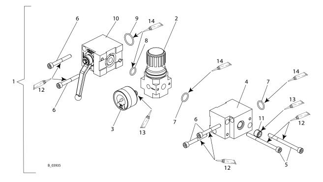
**Pos 3:** Screw in the pressure gauge until the white sealing ring is completely in the filter control valve. Thereafter continue turning the pressure gauge only to align the display scale.
