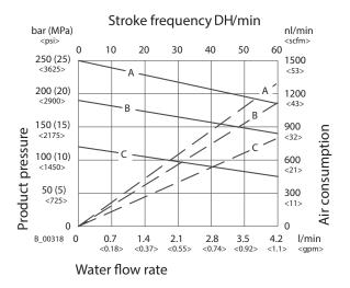
A = 7.1 bar (0.71 MPa; 103 psi) air pressure B = 6 bar; 0.6 MPa; 87 psi air pressure C = 4 bar; 0.4 MPa; 58 psi air pressure
