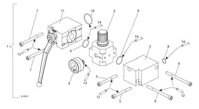
**Pos 4:** Screw in the pressure gauge until the white sealing ring is completely in the filter control valve. Thereafter continue turning the pressure gauge only to align the display scale.
