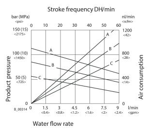
A = 8 bar (0.8 MPa; 116 psi) air pressure B = 6 bar; 0.6 MPa; 87 psi air pressure C = 4 bar; 0.4 MPa; 58 psi air pressure
