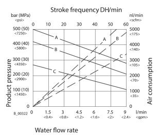
A = 7.1 bar (0.71 MPa; 103 psi) air pressure B = 6 bar; 0.6 MPa; 87 psi air pressure C = 4 bar; 0.4 MPa; 58 psi air pressure
