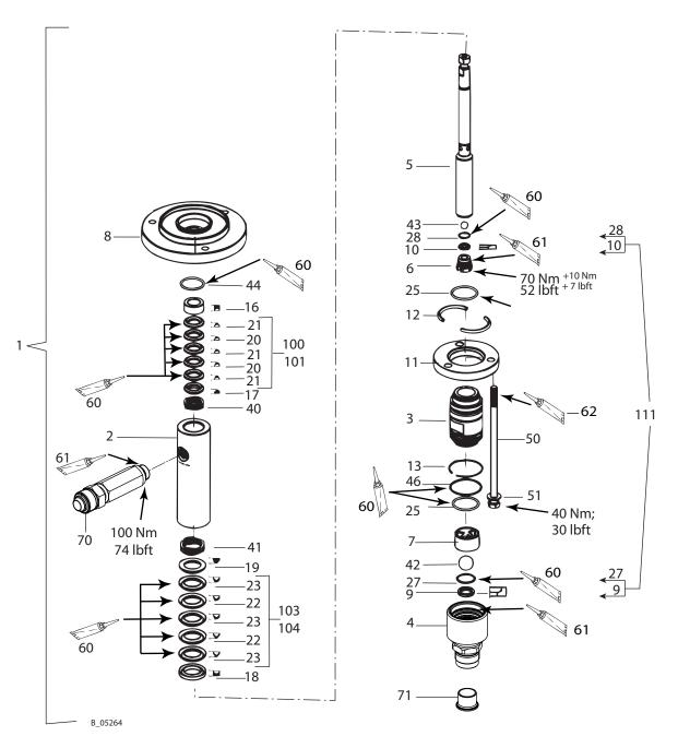
**Pos. 4** Tighten by hand on block. Use a standard wrench only if necessary. In this case use a spanner to hold pos. 3.
