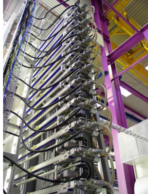
Fig.4 Multi-axis system with Z axes and rotary axis for each gun
