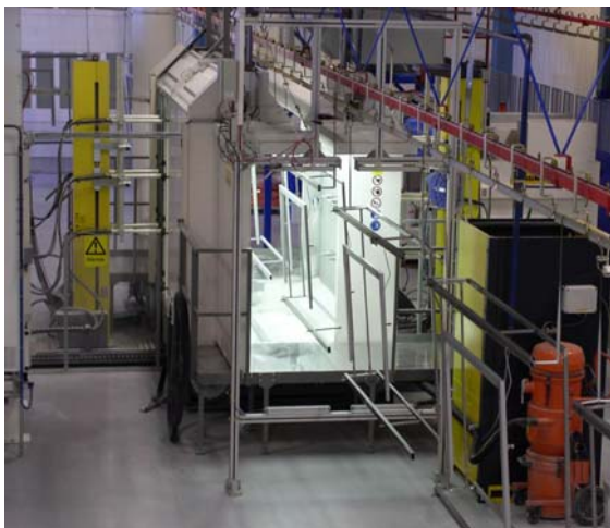
Fig. 1.: System with reciprocators and parts sensing in front of the booth
