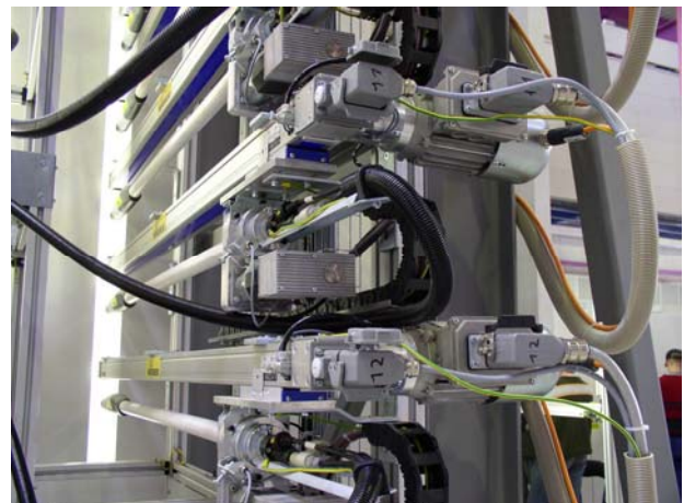
Fig. 2: Multi-axis system with Z axes and rotary axis for each gun
